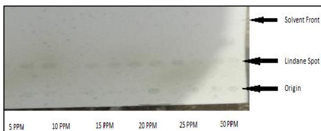
Fig. 7 TLC plate for estimating of different concentrations of lindane (5 ppm to 30 ppm) at 144 hours.
